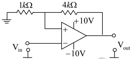
Which of the following correctly represents the output  $V_{out}$  corresponding to the input  $V_{in}$ ?
