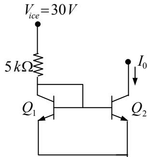
The current  $I_0$  (in mA) is \_\_\_\_\_ (upto two decimal places)
