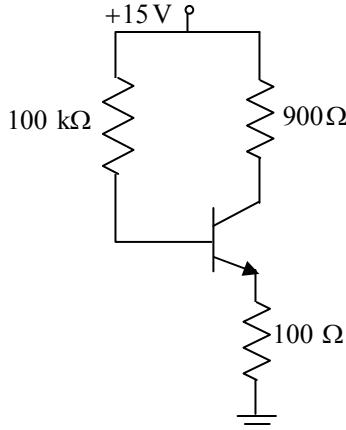
Which one of the following correctly represents the load line (collector current  $I_C$  with respect to collector-emitter voltage  $V_{CE}$ ) and Q-point of this circuit?
