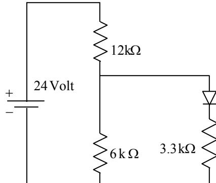
Solution: Let current through  $12k\Omega$  is  $I$  and through diode is  $I_D$
