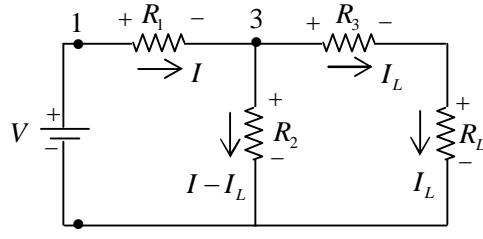
$$\text{Current through } R_1 \text{ is } I = \frac{V}{R_{eq,12}} \text{ where } R_{eq,12} = R_1 + \frac{R_2(R_3 + R_L)}{R_2 + (R_3 + R_L)}$$
