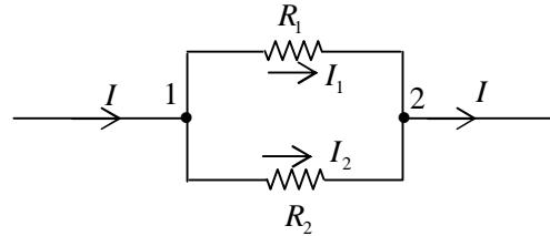
According to KCL at node 1 and 2:  $I = I_1 + I_2 \dots (i)$
