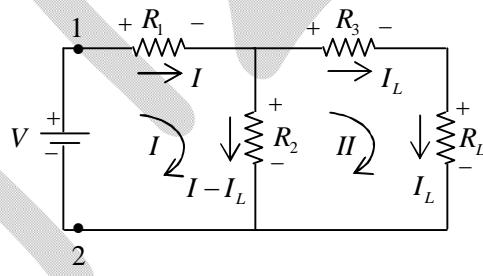
$$\text{In loop (I): } -V + IR_1 + (I - I_L)R_2 = 0 \dots (i)$$
