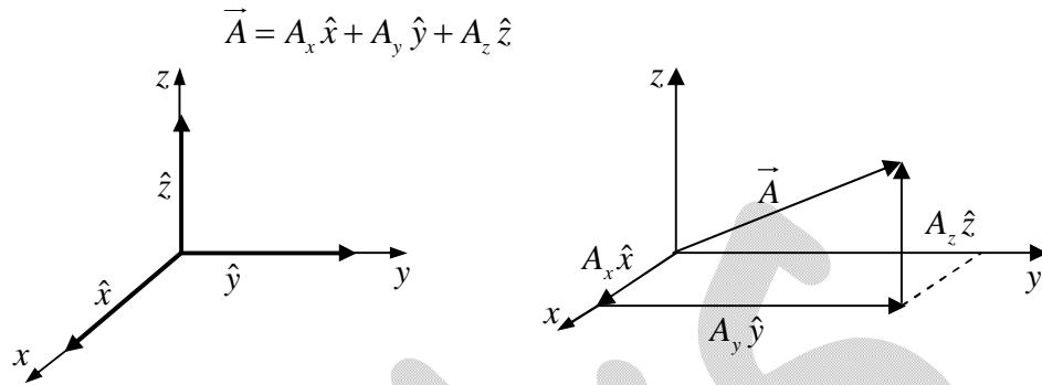
The numbers  $A_x$ ,  $A_y$ , and  $A_z$  are called component of  $\vec{A}$ ; geometrically, they are the projections of  $\vec{A}$  along the three coordinate axes.
