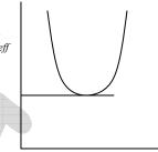
$k = \frac{d^2 V_{eff}}{dr^2}\bigg|_{r=r_0} = + \frac{3L^2}{mr^4} - \frac{2k}{r^3}\bigg|_{r=r_0} = \frac{3L^2}{m\left(\frac{L^2}{mL}\right)^4} - \frac{2k}{\left(\frac{L^2}{mL}\right)^3} = \frac{3m^3k^4}{L^6} - \frac{2m^3k^4}{L^6} = \frac{m^3k^4}{L^6}$
