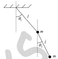
Solution: Let co-ordinate  $(x_1, y_1)$  and  $(x_2, y_2)$ .  $K.E. = \frac{1}{2}m(\dot{x}_1^2 + \dot{y}_1^2) + \frac{1}{2}m(\dot{x}_2^2 + \dot{y}_2^2)$
