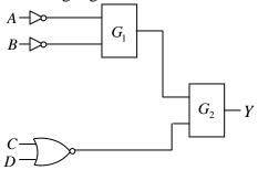
If  $Y = AB + \overline{CD}$ , the gates  $G_1$  and  $G_2$  must, respectively, be
