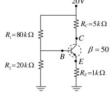
If the resistor  $R_2$  is disconnected, the voltages  $V_B$  at the base and  $V_C$  at the collector change as follows.
