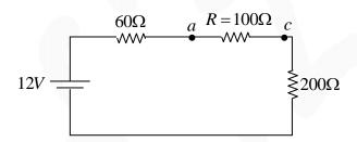
Voltmeter is connected across point ac in parallel.
