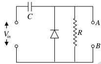
If the signal has time period  $\tau_s$  and the circuit has a natural frequency  $\tau_{RC}$ , then in the case when  $\tau_s << \tau_{RC}$ , the steady-state output will resemble
