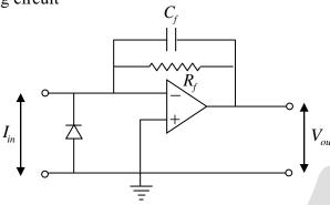
It is given that  $C_f = 100 \ pF$ , and for  $l_{in} = 50 \ nA$  D.C,,  $V_{out} = 1V \ D.C$ ,. Therefore, the bandwidth of the above circuit is
