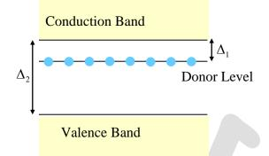
If the band gap between donor level and conduction band is  $\Delta_1$  and that between conduction and valence band is  $\Delta_2$  where  $\Delta_2 \Box \Delta_1$ , which of the following figures depict the qualitative features of the resistance (*R*) - vs-temperature (*T*) graph of the semi-conductor?
