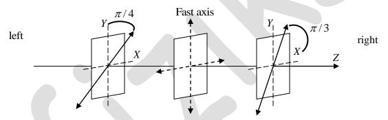
The apparatus consists of (from left to right) a polariser with transmission axis at  $\frac{\pi}{4}$  w.r.t. y-axis, followed by a quarter-wave plate with fast axis along the y-axis and finally, a polariser with transmission axis at  $\frac{\pi}{3}$  about the x-axis.
