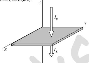
A plane radio wave of intensity  $I_0$  and frequency 29.5 *MHz* propagates in vacuum along the negative *z*-axis and strikes the metal foil at normal incidence.
