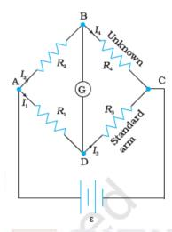
The null-point condition is given by  $\frac{R_1}{R_2} = \frac{R_3}{R_4}$  using which the value of one resistance can be determined, knowing the other three resistances.
