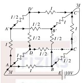
**Question 13:** Determine the current in each branch of the network shown in figure below.
