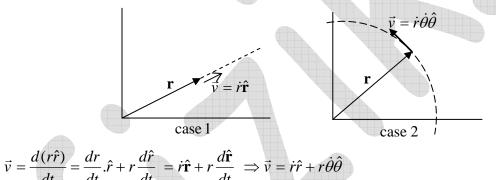
where  $\dot{r}$  is radial velocity in  $\hat{r}$  direction and  $r\dot{\theta}$  is tangential velocity in  $\hat{\theta}$  direction as shown in figure and the magnitude to velocity vector  $|v| = \sqrt{\dot{r}^2 + r^2 \dot{\theta}^2}$
