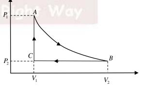
(D) Total change in internal energy during the entire process is  $\frac{5}{2}P_2(V_2-V_1)$
